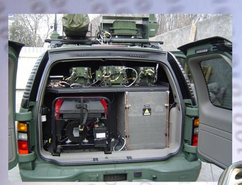
The system supports voice and data communication requirements while "On-the-Move" or while deployed in a "Static" location. A comfortable, ergonomic and spacious radio operator compartment provides convenient access and operation of the communication assets. Deployed operation is accomplished using the RF-5800R-RC001 Field Wire Remote System, which supports remoting the full range of functionality of the Falcon II radios over a single pair of field wire at distances up to 3 km.
