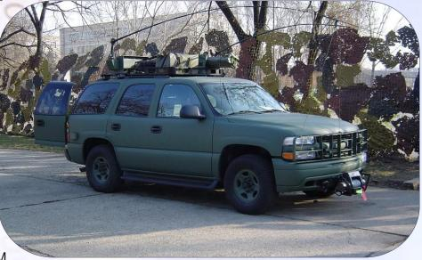
A General Motors (GM) Light Service Support Vehicle (LSSV) four-wheel drive vehicle provides the common mobile platform for the communications system. The vehicle is custom equipped with AC and DC power distribution and conversion systems for the communications and support equipment. A power monitor and control panel provides convenient access for the operator to the system power functions. The
