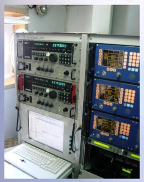
The management and control of the APCOS 4000 is performed by COSYMA (COmmunications SYstem MAnagement). Specific network equipment is provided for COSYMA functionality. This includes a server with RAID (Redundant Array of Inexpensive Disks), as operator (supervisor) console and CMT (Communication Management Terminal) which provide overall system and network management and ACP 127 SAMMS (Secure Automatic Military Messaging System) and two SAMMS laptop workstations.
